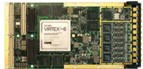
Innovative X6-250M PCI Express PMC module with RF digitizing front-end
