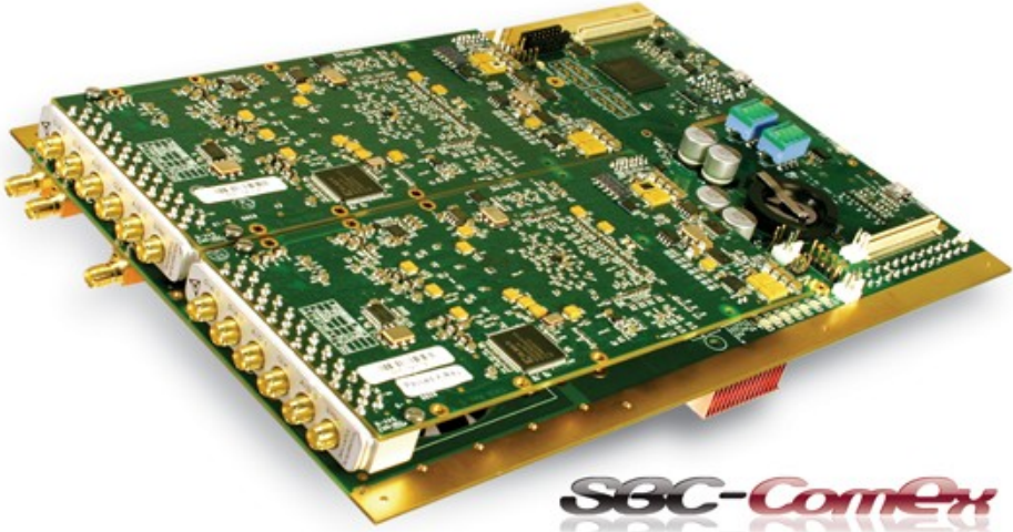
Figure 2. SBC-ComEx Carrier Board with Dual XMC modules installed
