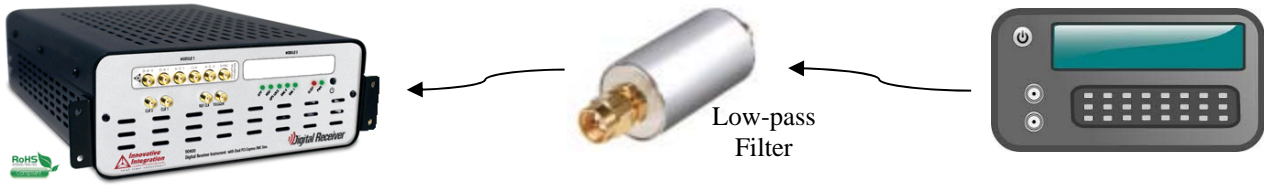
Figure 6. Test environment; anti-aliasing filter is used between the digital receiver and functional generator
