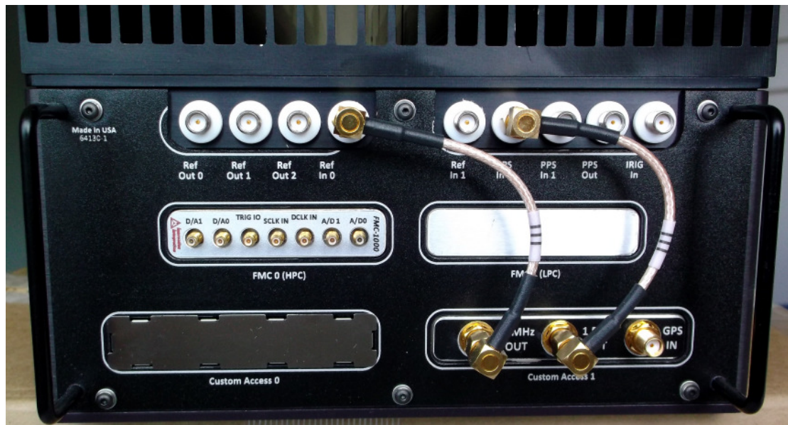
Front of ePC-K7 showing analogue inputs and GPS connections
