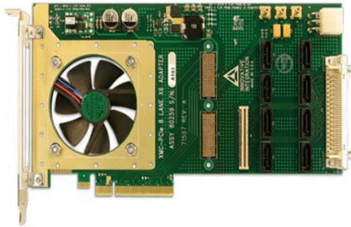
Optional 8-Lane XMC to PCI Express Adapter Card, P/N 80259-0
