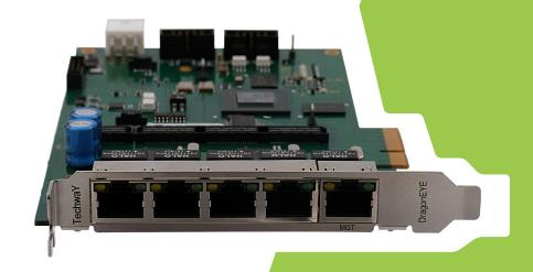
Machine Vision applications process an ever-increasing amount of information that must not be limited by the processing capabilities of computers. To exceed this bandwidth limit, TECHWAY has developed a range of multi-camera acquisition boards equipped with a processor unique of its kind.
