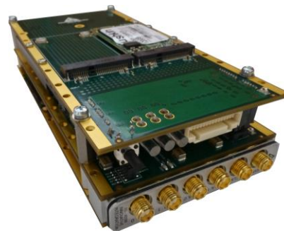
Figure 5. Rear isometric view of SBC-Nano system in a chassis.
