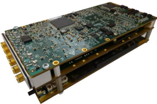
Figure 6. Top view of SBC-Nano electronics stack: XMC module (X6-400M module is shown), SBC-Nano Carrier Board and SBC-Nano Extension Board.
