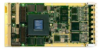
The XA-AWG is an XMC IO module featuring eight 16-bit, 250 MSPS DAC channels designed for cellular base stations, diversity transmit, and wideband communications.
