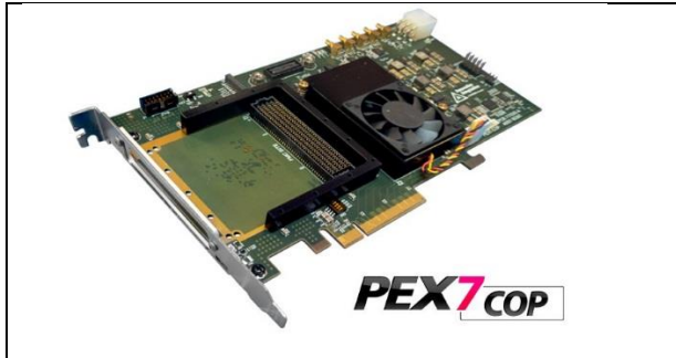
Figure 4. PEX7-COP Carrier board with Kintex 7 FPGA
