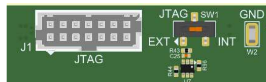
Figure 4. JTAG Mode Selection Switch SW1 and External JTAG Header J1
