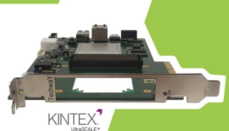
The new PFP-IV is a multi-purpose PCIe platform with FMC+ site based on the powerful Xilinx Kintex UltraScale+ FPGA. This board is dedicated for extreme high-speed applications such as 100 GbEth communications, 4/6 GHz ADC/DAC, ARINC 818, AURORA, JESD, sFPDP, etc.
