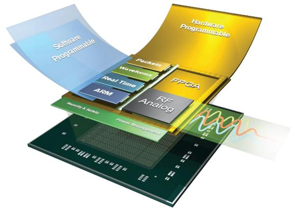
The AMD Zynq® UltraScale+™ RFSoc integrates RF-class A/D and D/A converters into the Zynq® FPGA fabric and multi-core ARM processor subsystem, creating a multi-channel data conversion and processing solution on a single chip.
